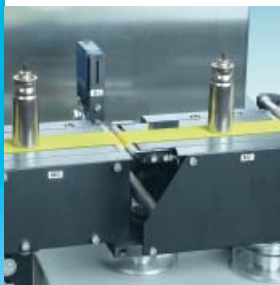
Ultra-lightweight weighing conveyor – core of the XS1 system
